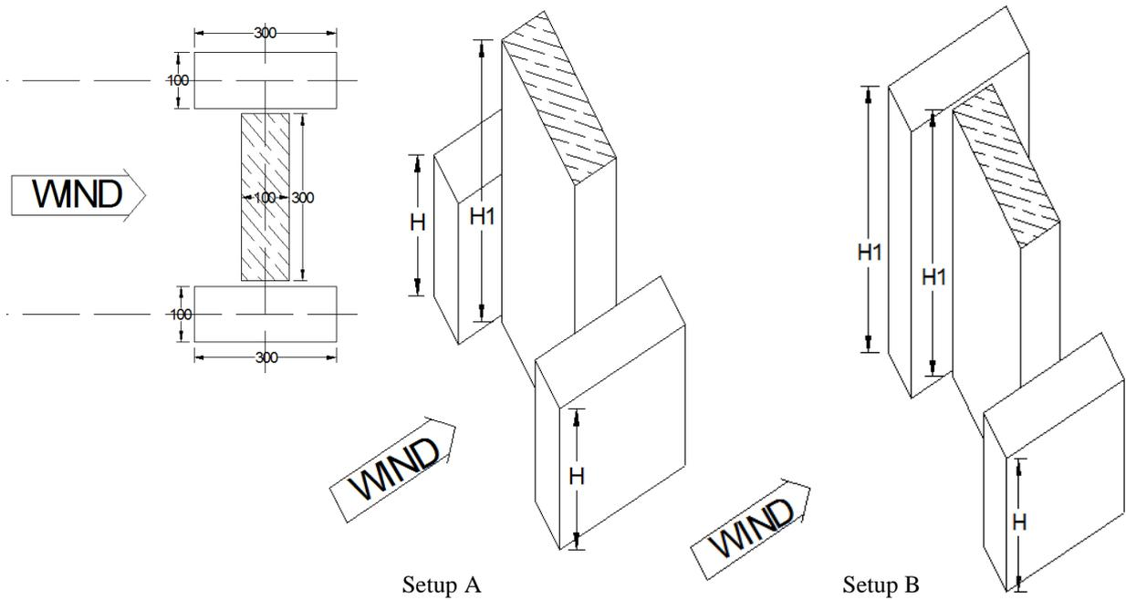
**Figure 1.** Plan and isometric view of the different arrangements for experimentation (All Dimensions are in mm).
