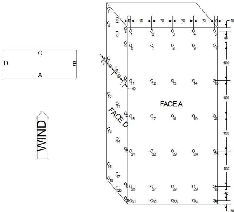
**Figure 2.** Plan and isometric view of principal building showing the location of pressure tapping points.
