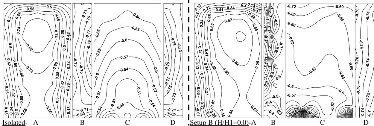
Figure 3. Contour diagrams for distribution of mean wind pressure coefficients.
