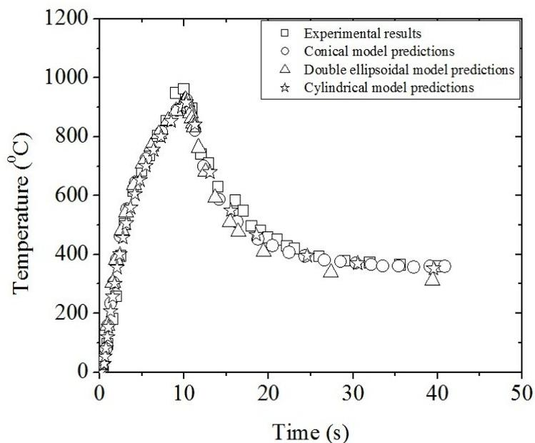
Fig. 1. Comparison of the results of temperature vs. time at 4.5 mm distance from melt zone.
