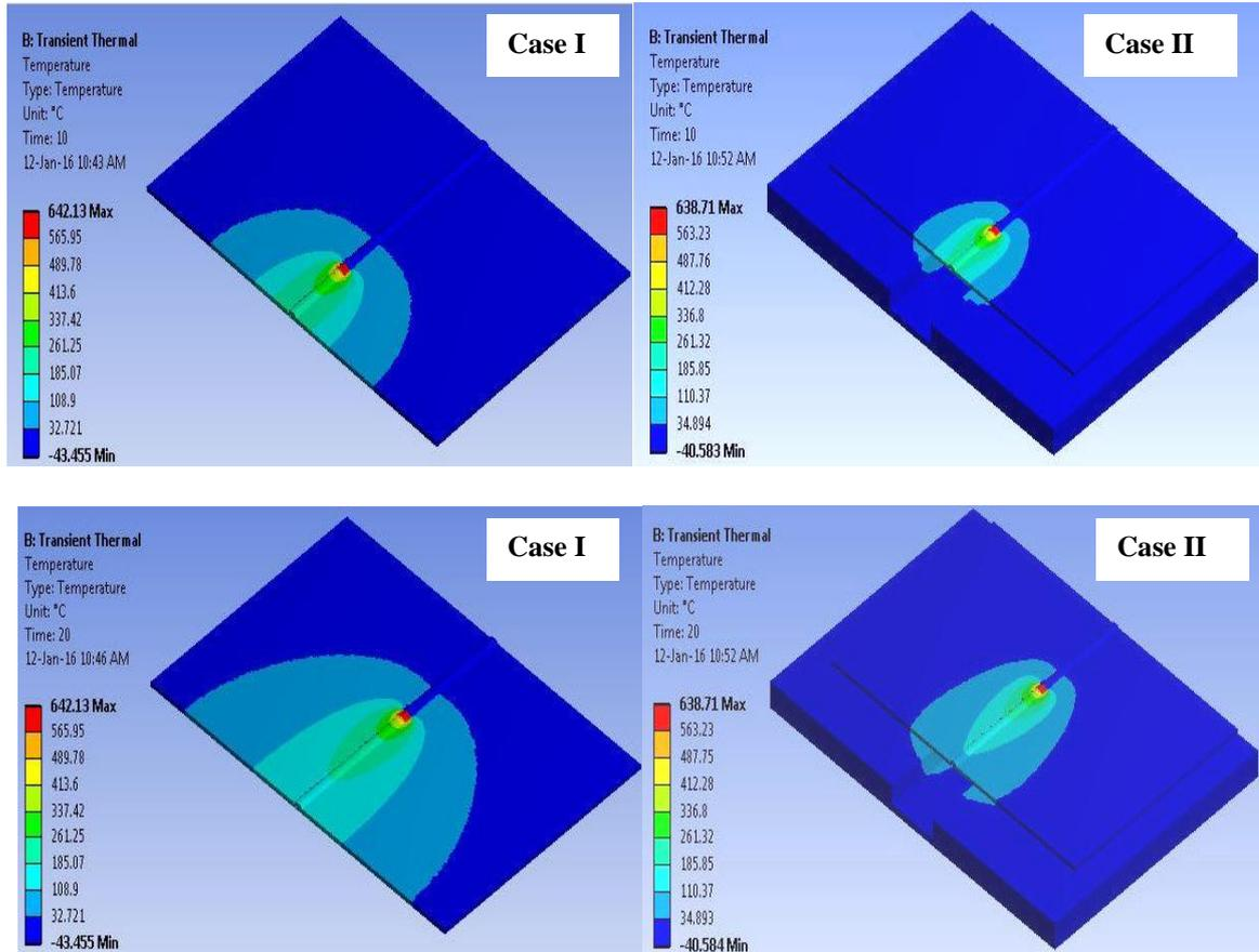
**Figure 1.** Numerical results for transient temperature in case I and case II at time steps of 10s and 20s in GMAW welding.
