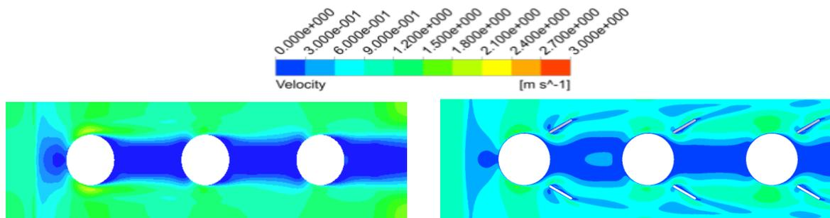
**Fig.1:** Velocity contours for baseline, rectangular vortex at 30° placed behind the tube
