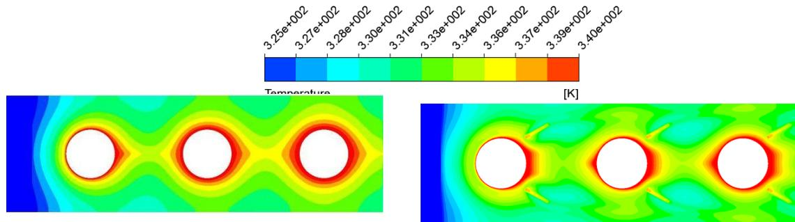
**Fig. 2:** Temperature contours for baseline, rectangular vortex at  $30^\circ$  placed behind the tubes
