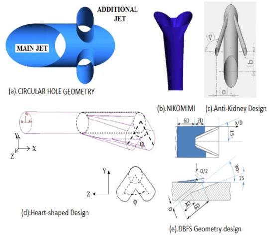
Figure 2: Different film cooling hole Geometries proposed in recent studies.
