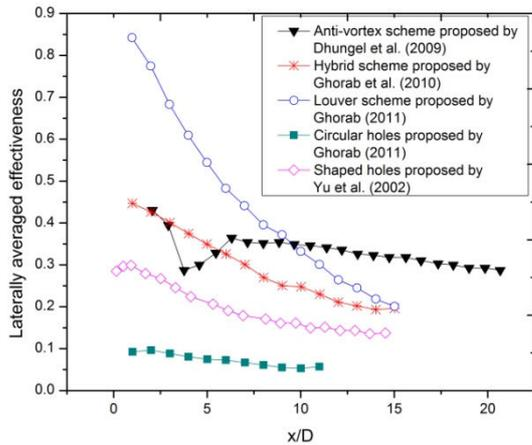
Figure 1: Comparison of various schemes at blowing ratio of 1.
