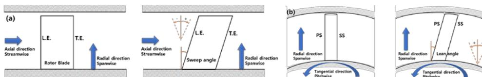
Fig. 1 Definition of (a) blade sweep and (b) blade lean
