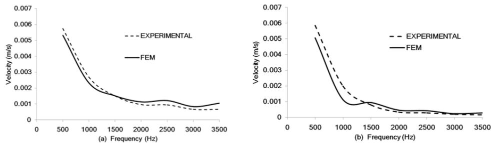
**Fig. 1.** Velocity Responses for Plate 1 and Plate 2 (Case -1)
