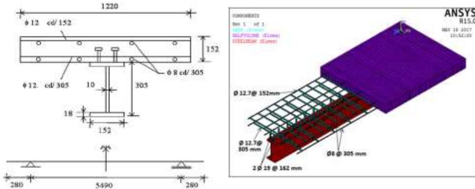
**Figure 1.** Cross-section of a typical composite section and its finite element model
