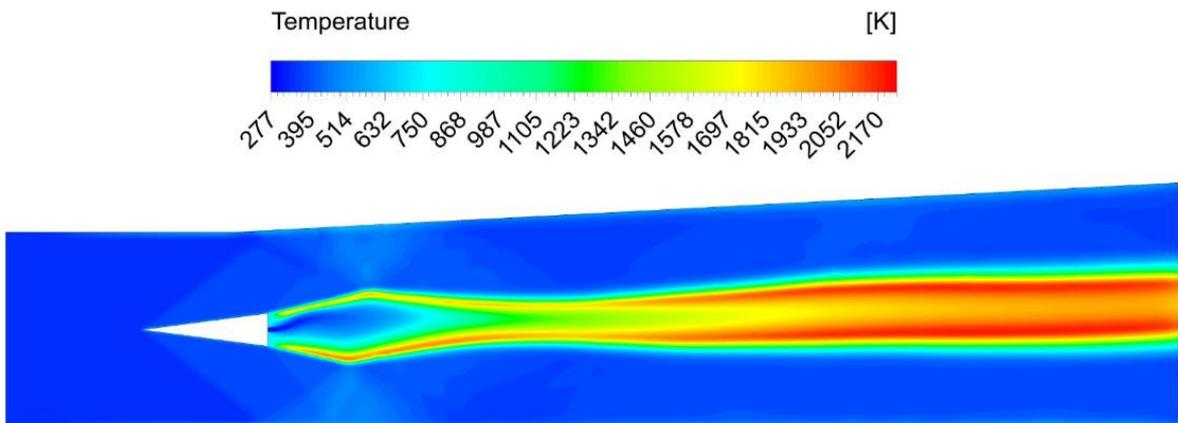
Fig. 4: Temperature Contours (15 degree symmetric strut)
