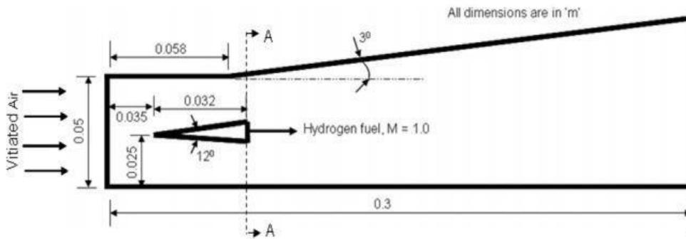
Fig. 3: Geometry of Scramjet Combustor
