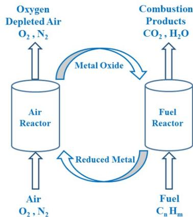
Figure 1. Schematic of a chemical looping combustion system.
