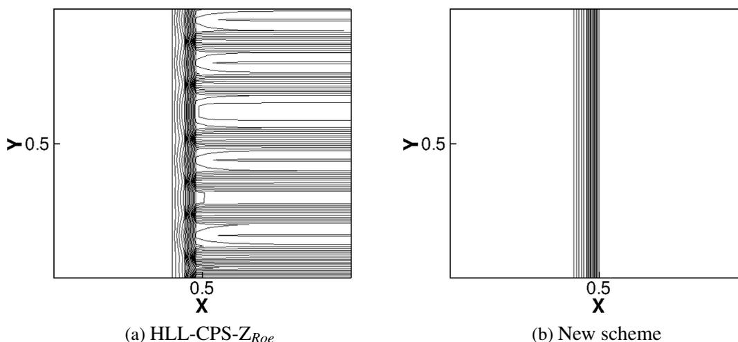
Figure 1: Density contours for M=7 standing shock instability problem.
