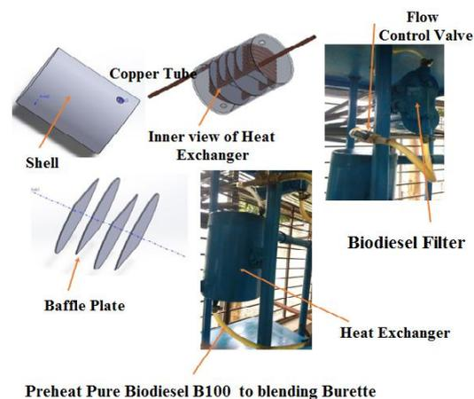
Fig. 1: Three dimensional sectional and photographic view of preheating assembly device.
